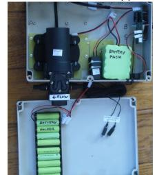
the battery holder in the lid and connect that to the PCB. This will be either 10 or 20 batteries. Be careful to ensure all the batteries are the right way around and not to strain the connecting wires.
